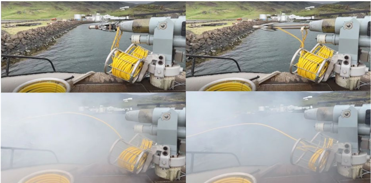
Image 12 - A new type of firing line basket (line follows the direction of the harpoon gun)
