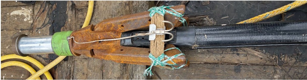
Image 19 - Harpoon with a harpoon grenade hook
