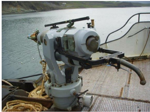
Image 4 - 90 mm Kongsberg whaling gun with a loaded harpoon
