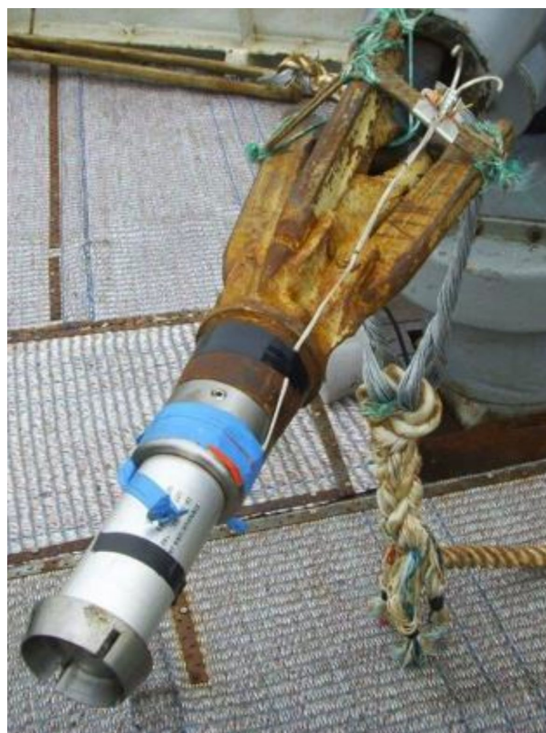
Image 6 - A harpoon and a Hvalgranat-99 grenade with a hook
